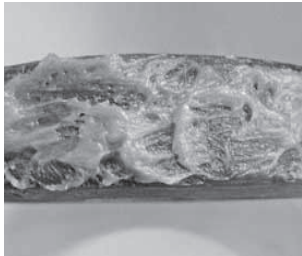
Improperly Lubricated Gasket
